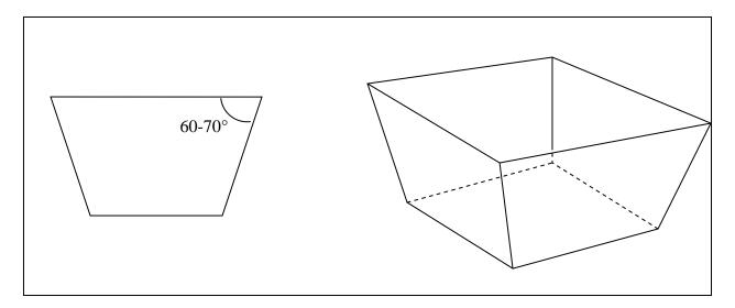
The most important thing the students can do to create solar ovens that will work well is to make sure there are no places where air can flow out of the interior of the oven. If the hot air can just flow out of an open space in the oven, the insulation will not be able to keep the heat in.
